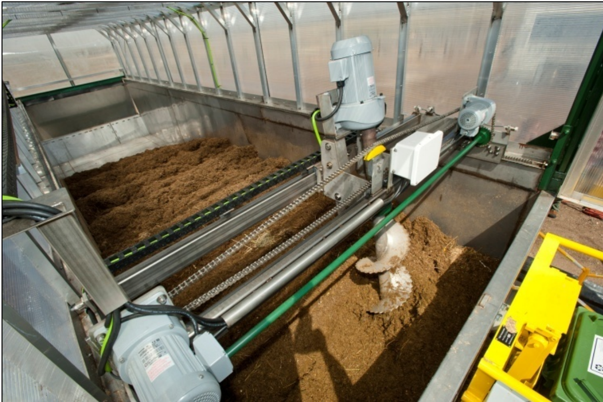
The CSU in-vessel composter processes up to 2,000 pounds/ day of food waste and animal bedding
